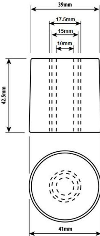
Suitable for Refrigeration, Water, Oil, Air-conditioning, gas, Air installations and other plant and machinery where solenoid valves require opening and closing manually. The Solenoid Valve Operating Magnet has been designed and manufactured to solve the problem of how to operate Solenoid Valves when a system is not under power. The Magnet is the same shape and size of a large cotton reel and, when placed on top of a Solenoid Valve with the coil removed, it causes the armature to open or close.
